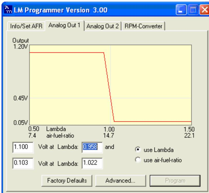
This shows the analog output voltages versus Lambda for one of the two analog outputs. The graph display is automatically scaled to the selected voltages. For each output you can specify a
