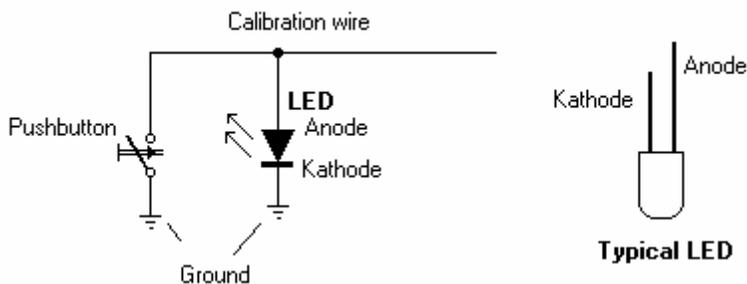
Any color LED can be used. A typical LED has 2 wires called Anode and Kathode. The Kathode side is the shorter of the 2 wires. It is connected to Ground. The Anode side will be connected to the calibration wire.
