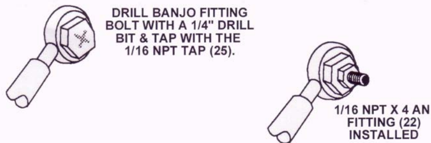
Figure 8 Schematic of "Drilled Out" Banjo Fitting
