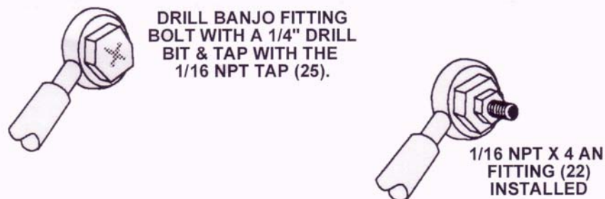
Figure 8 Schematic of "Drilled Out" Banjo Fitting
