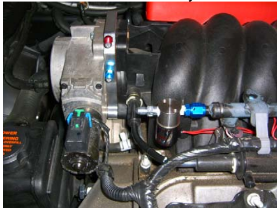
LS6 engine shown, same fuel rail setup for LS2
