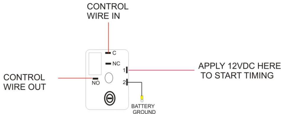
You can use this timer to also disconnect terminals! Terminals “C” and “NC” are connected inside the relay with no power applied to terminal “1”. Apply 12V to Terminal 1 and after the time delay relay counts down and turns on... terminal “C” and Terminal “NC” are disconnected inside the relay, just like flipping a switch off. You can run 12v though these terminals, you can run a ground though them etc...
