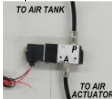
Port labeled "P" goes to the air tank/supply, port labeled "A" goes to the air cylinder/air cylinder, port labeled "EA" is the exhaust and this port is left open.
