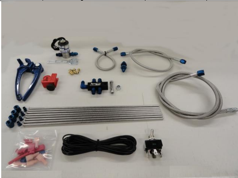
Figure 1. Black Widow EFI BIKE Kit Components
