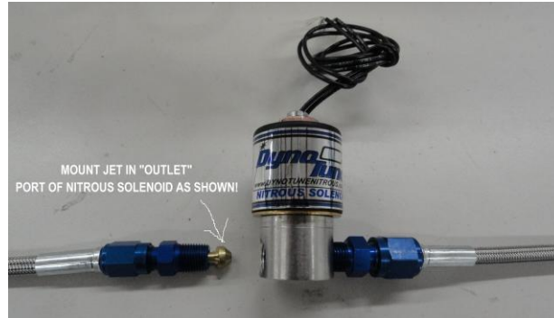
Spray bar installation
